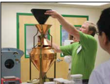
Pat Kehoe from the ND Grain Inspection Service demonstrates the Boerner grain divider.
