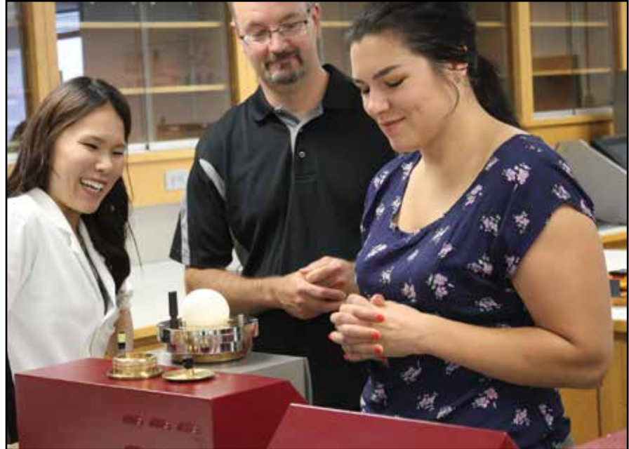
Natsuki Fujiwara, NCI Food Scientist, assists two participants as they run a test for dough strength on the Chopin Alveograph.
