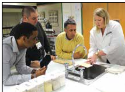
Rachel Carlson, NCI Food Technologist, demonstrates the Pekar Slick Test that compares a flour sample's color against a standard sample.
